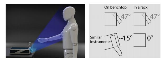
Figure 2.2: TiltView<sup>™</sup> angle comparison
