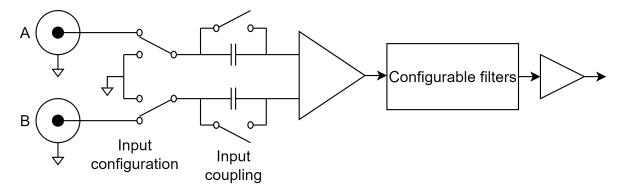
Figure 4.5: Module equivalent diagram
