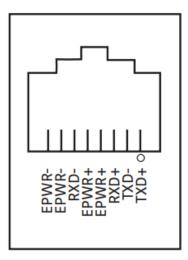
Figure 7.5: Ethernet connector
