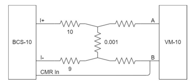
In external CMR mode, the BCS-10 will adjust the I+ and I- outputs to produce 0 V at the CMR sense point, which has been connected to the VM-10 B input. Now the VM-10 is presented with only 100  $\mu$ V of common mode voltage, significantly reducing the error.
