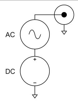
Figure 4.1: Module equivalent diagram
