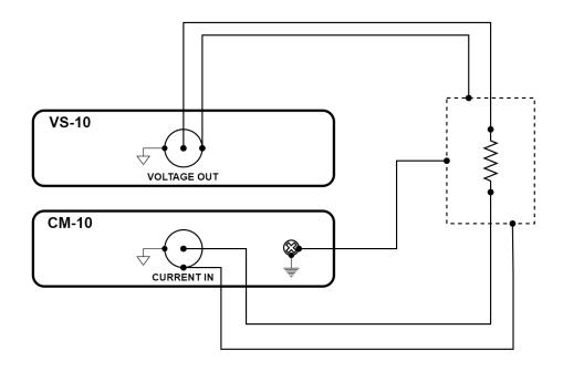
Figure 3.38: Resistance measurement using a VS-10 module and a CM-10 module
