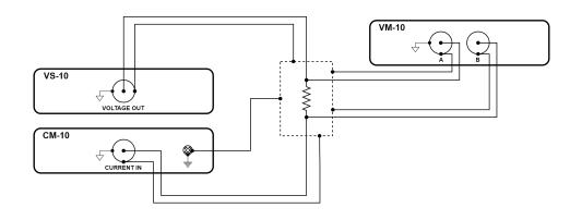
Figure 3.39: Resistance measurement using VS-10, CM-10, and VM-10 modules
