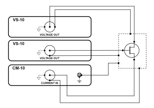
Figure 3.41: FET transistor measurement using VS-10, CM-10, and VM-10 modules
