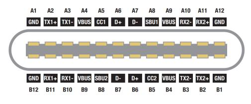
Figure 7.4: USB Type-C<sup>™</sup> connector
