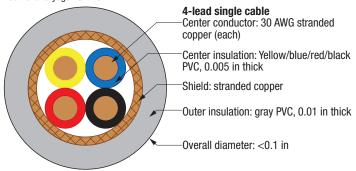
Rated temperature: -20 °C to 80 °C Thermal conductivity (300 K): 400 W/(m·K)
