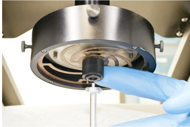
Figure 2-34. Attaching the Sample Tail
