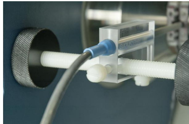
Figure 2-20. Gaussmeter Probe Holder Installation
