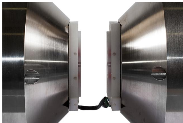
Figure 2-18. Typical Model 740 ESC large coils with EM7-4P pole caps on the Model EM7-HV magnet
