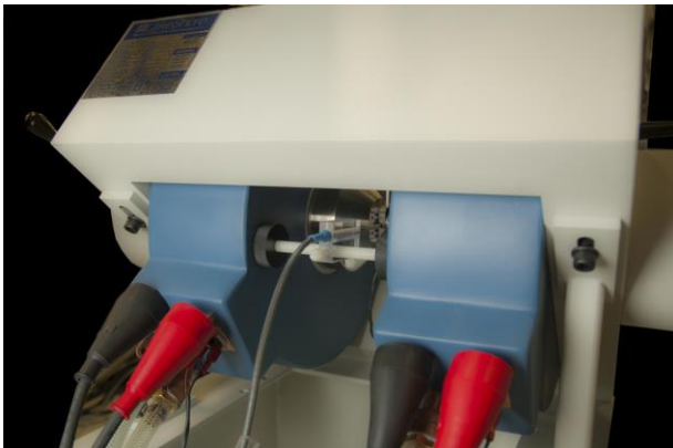
Figure 2-20. Gaussmeter Probe Holder Installation
