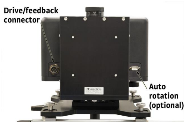
Figure 2-16. Typical VSM Drive Connections
