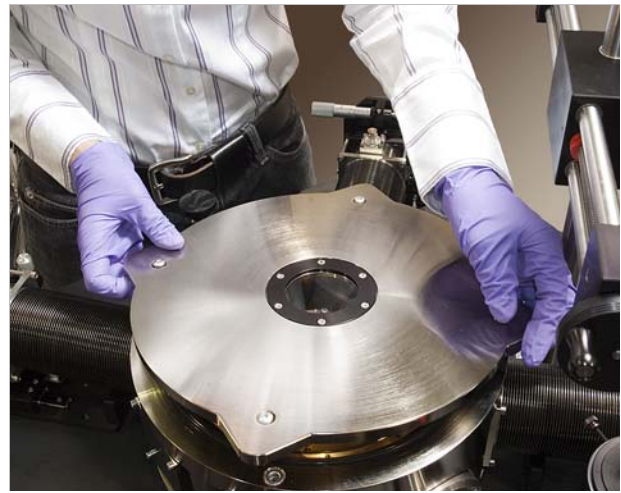
FIGURE 4-3 Left: Vacuum isolation valve on the probe station; Right: CPX-VF probe station vacuum chamber lid removal
