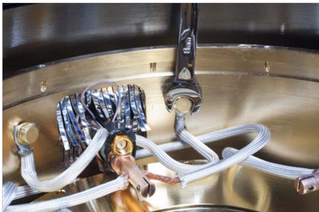
FIGURE 5-5 Left and Right: Use a wrench to remove the probe mount braids from the radiation shield
