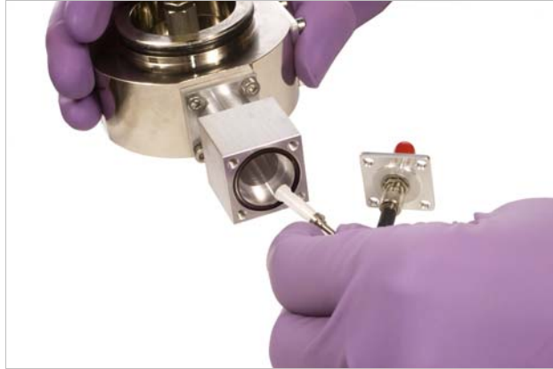
FIGURE 5-19 Insert the optical fiber tip into the feedthrough extension
