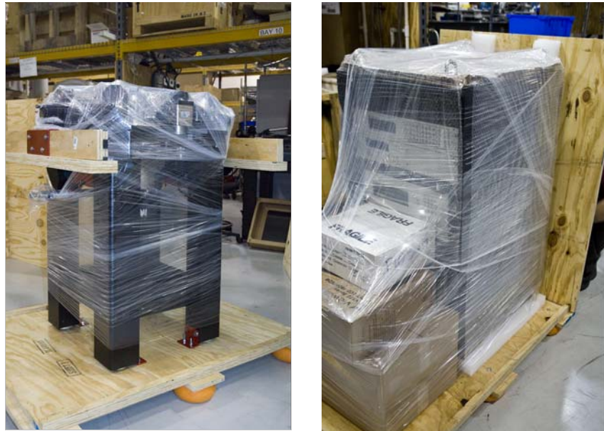
FIGURE 3-3 If you suspect damage, take a photo of the packed shipment, specifically damaged areas Left: Probe station; Right: Console and accessories
