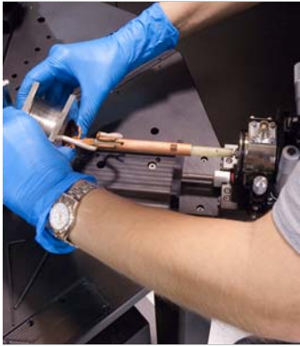
FIGURE 5-12 Left: Placing the bellows onto the probe arm base; Middle: Attach the bellows to the z-axis stage; Right: Spacers between the bellows and the z-axis stage
