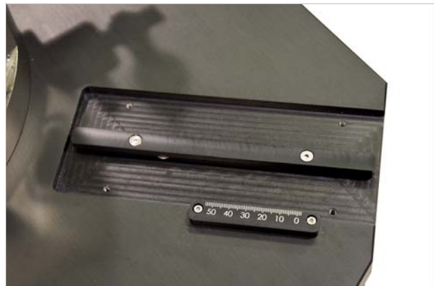
FIGURE 5-1 Left: Remove the screws from the slide insert; Right: Secure the slide insert to the arm stage location
