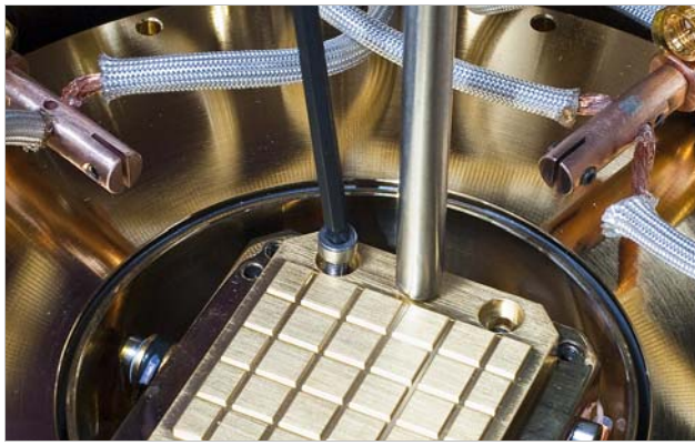
FIGURE 4-6 Left: Fastening the sample holder onto the sample stage; Right: Connecting the signal cable on a triaxial or coaxial sample holder
