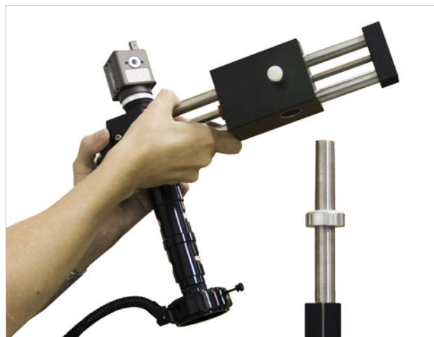
FIGURE 3-9 Installing the horizontal boom onto the vertical post
