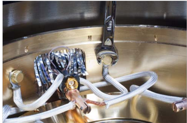
FIGURE 5-4 Left: Slide the spade lug under the hex screw head and washer; Right: Tighten the hex screw to attach it to the radiation shield
