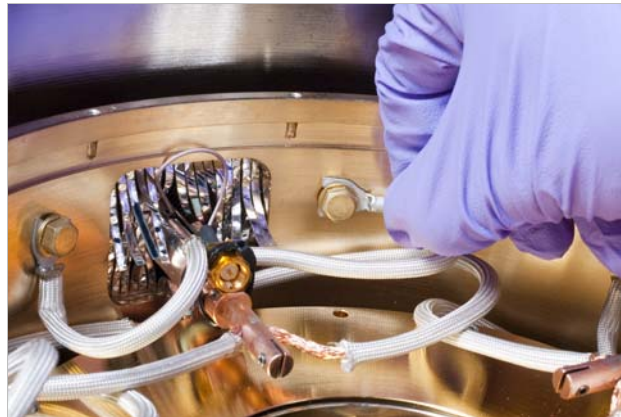
FIGURE 5-5 Left and Right: Use a wrench to remove the probe mount braids from the radiation shield
