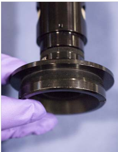
FIGURE 3-11 Left: Installing the ring light onto the adapter; Middle: Tighten the ring light thumbscrews; Right: Fiber optic cable attached to the light source
