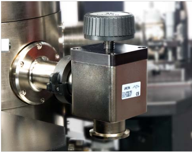
FIGURE 4-3 Left: Vacuum isolation valve on the probe station; Right: CPX-VF probe station vacuum chamber lid removal
