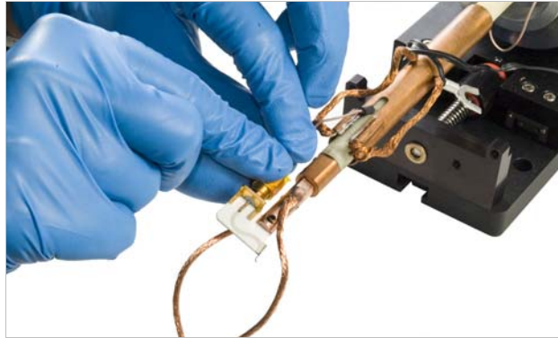
FIGURE 3-25 Disconnect the SMA
