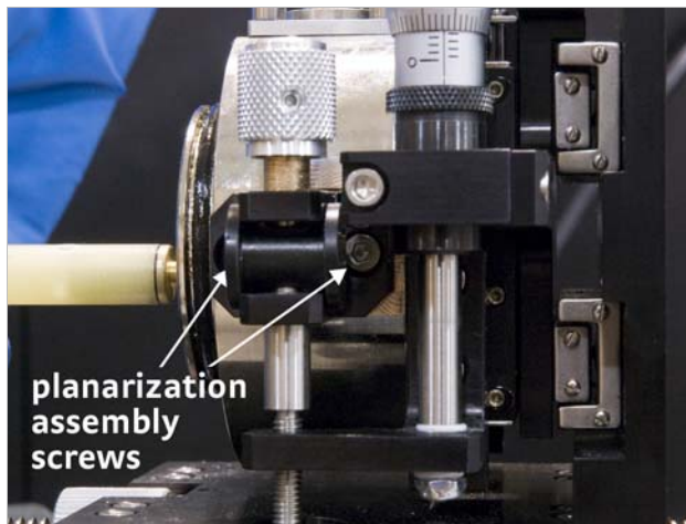
FIGURE 5-11 Left: Securing the planarization assembly to the probe arm base; Right: Taping the cable to the probe arm
