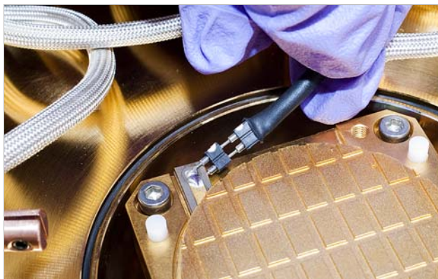
FIGURE 4-4 Left: Disconnecting the triaxial sample holder; Right: Cable plug left out after disconnecting
