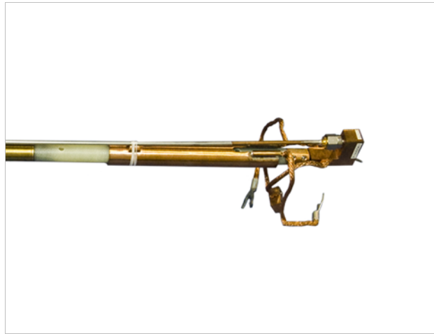
FIGURE 3-30 Microwave probe threaded onto a semirigid cable
