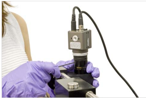
FIGURE 6-8 Loosening the camera rotating joint to adjust the camera image orientation
