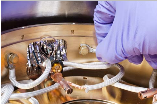
FIGURE 5-4 Left: Slide the spade lug under the hex screw head and washer; Right: Tighten the hex screw to attach it to the radiation shield
