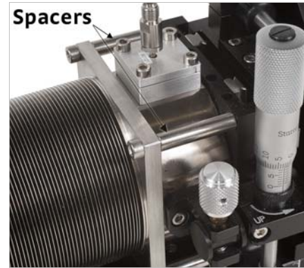
FIGURE 5-12 Left: Placing the bellows onto the probe arm base; Middle: Attach the bellows to the z-axis stage; Right: Spacers between the bellows and the z-axis stage
