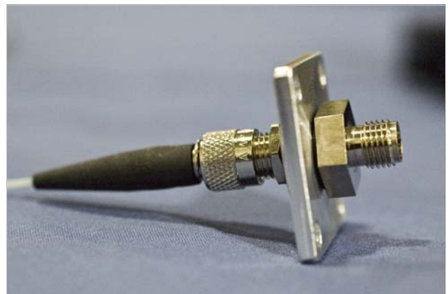
FIGURE 5-18 Left: Attaching the feedthrough extension to the probe arm base; Right: The nut between the cable and the flange—SMA style shown
