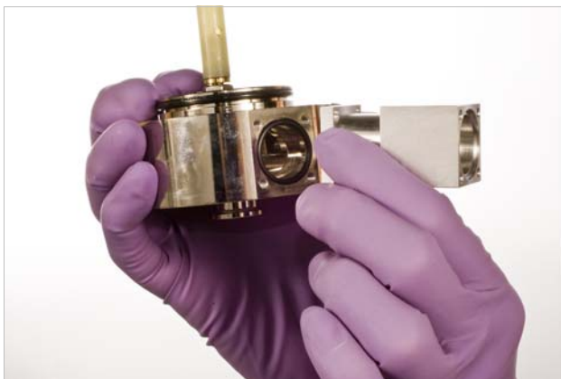
FIGURE 5-18 Left: Attaching the feedthrough extension to the probe arm base; Right: The nut between the cable and the flange—SMA style shown
