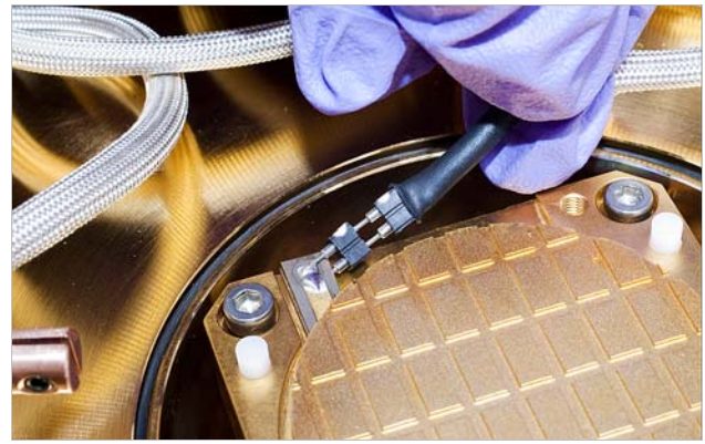
FIGURE 4-6 Left: Fastening the sample holder onto the sample stage; Right: Connecting the signal cable on a triaxial or coaxial sample holder
