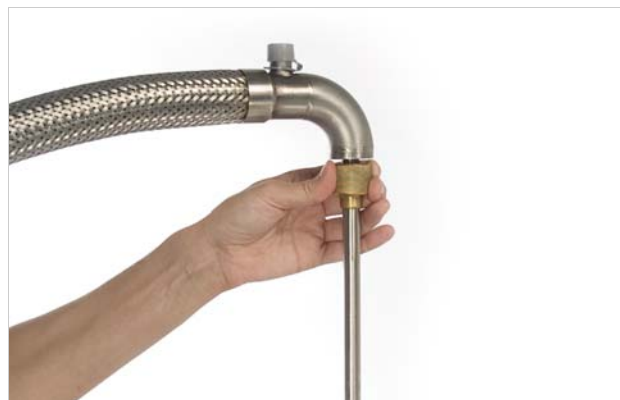
FIGURE 4-13 Left: Bayonet compression fitting on the transfer line shoulder; Right: Opening the foot valve
