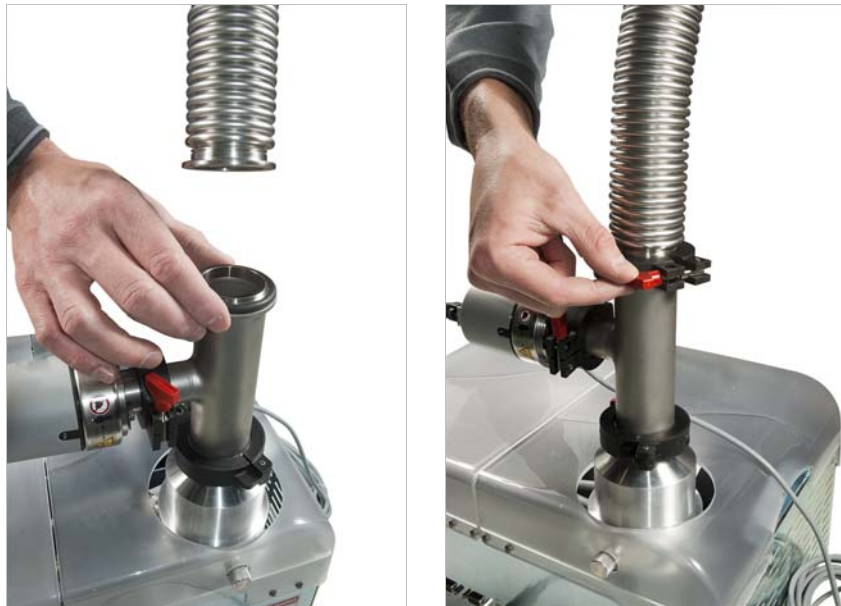
FIGURE 3-15 Install the vacuum line to the pump
