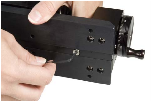
FIGURE 5-1 Left: Remove the screws from the slide insert; Right: Secure the slide insert to the arm stage location
