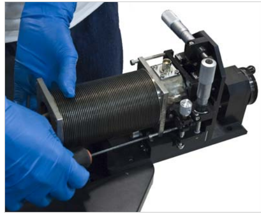
FIGURE 5-24 Left: Thread the nut onto the bottom of the shaft; Right: Tighten the four long horizontal M4 screws
