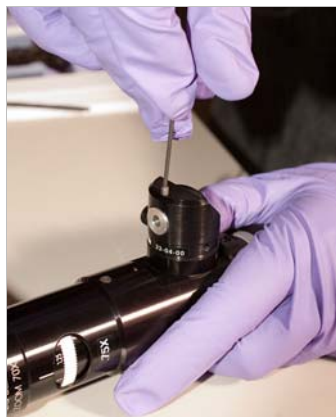
FIGURE 3-12 Left: Loosen the set screw on the fiber optic cable fitting; Middle: Remove protective fitting; Right: Insert the fiber optic cable
