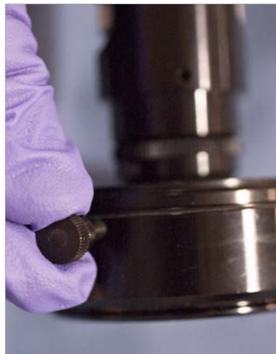
FIGURE 3-11 Left: Installing the ring light onto the adapter; Middle: Tighten the ring light thumbscrews; Right: Fiber optic cable attached to the light source
