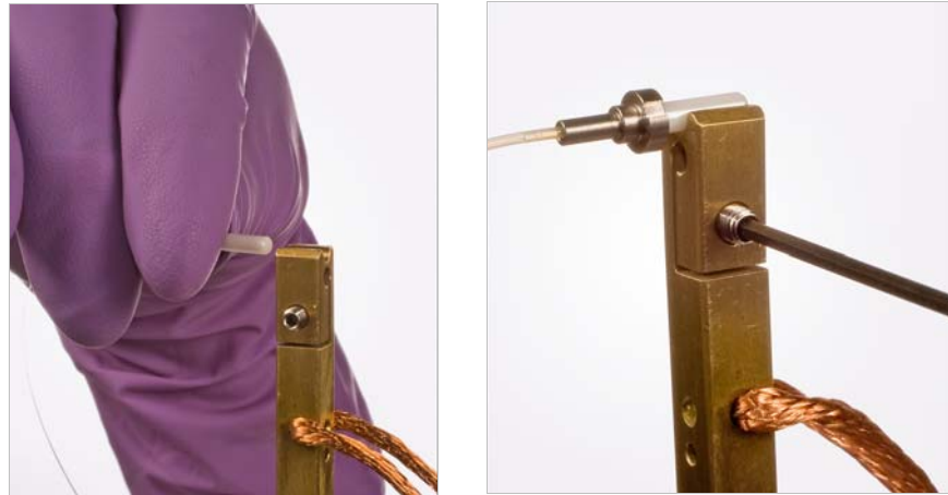
FIGURE 5-20 Left: Inserting the optical fiber tip into the opening in the probe mount; Right: Securing the optical fiber tip by tightening the M3 screw
