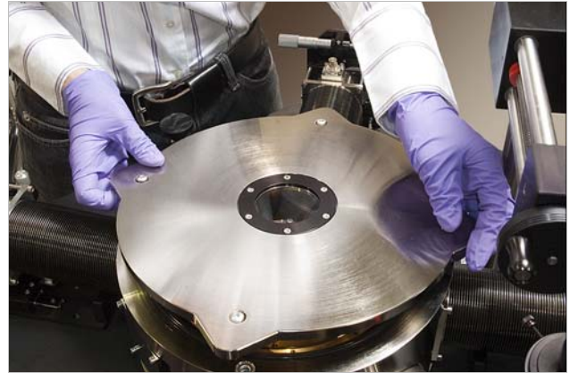
FIGURE 4-8 Left: Placing the o-ring in the chamber groove; Right: Placing the chamber lid onto the o-ring
