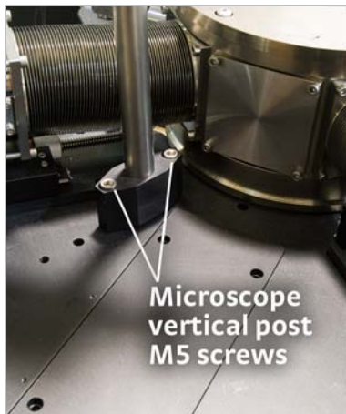
FIGURE 3-8 Left: Installing the microscope vertical post; Middle: Four M3 mounting screws on the vertical post; Right: Attaching the microscope to the horizontal boom
