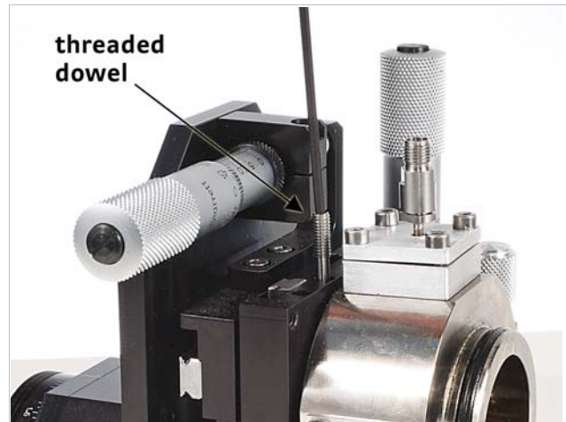
FIGURE 5-9 Left: Loosen the two screws holding the planarization assembly to the probe arm base; Right: Pull out the threaded dowels
