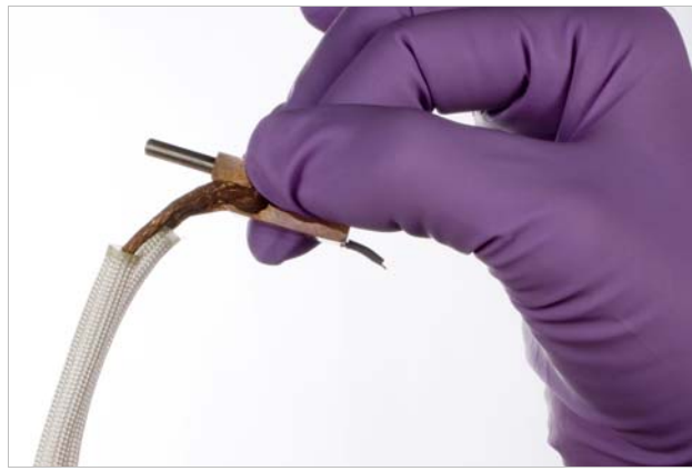
FIGURE 3-28 Proper handling of a microwave probe
