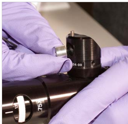
FIGURE 3-12 Left: Loosen the set screw on the fiber optic cable fitting; Middle: Remove protective fitting; Right: Insert the fiber optic cable
