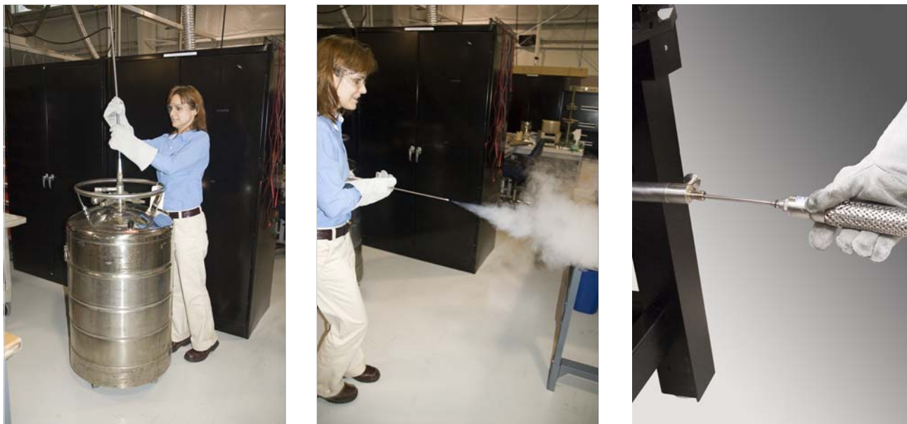
FIGURE 4-14 Left: Inserting the transfer line into the Dewar; Middle: Plume indicating the process of precooling the transfer line is complete; Right: Inserting the transfer line into the bayonet on the probe station
