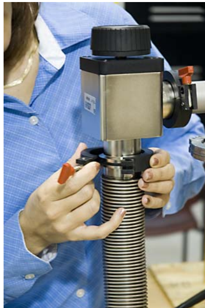
FIGURE 3-16 Use the clamp provided to attach the vacuum line to the probe station
