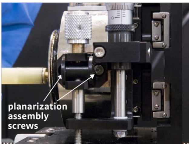
FIGURE 5-9 Left: Loosen the two screws holding the planarization assembly to the probe arm base; Right: Pull out the threaded dowels
