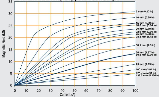
EM7-HV 76 mm (3 in) pole face field plot
