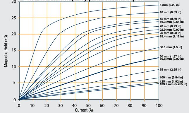
EM7-HV 102 mm (4 in) pole face field plot
