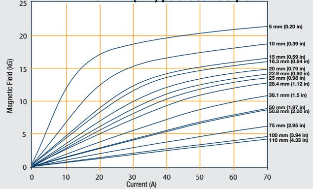
EM7-HV 51 mm (2 in) pole face field plot
