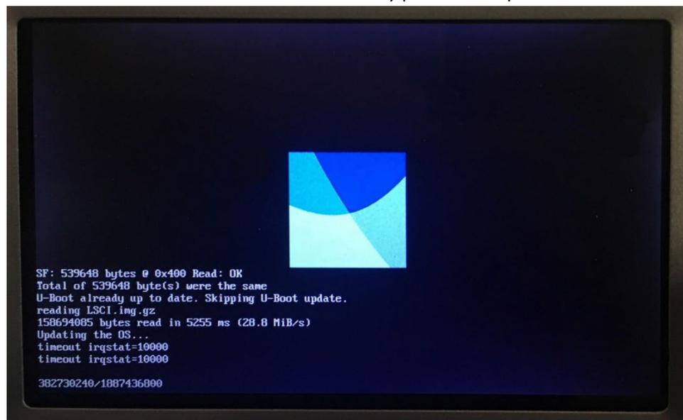
5. Once the OS is updated, the instrument will automatically install the firmware that is specific to that instrument.
