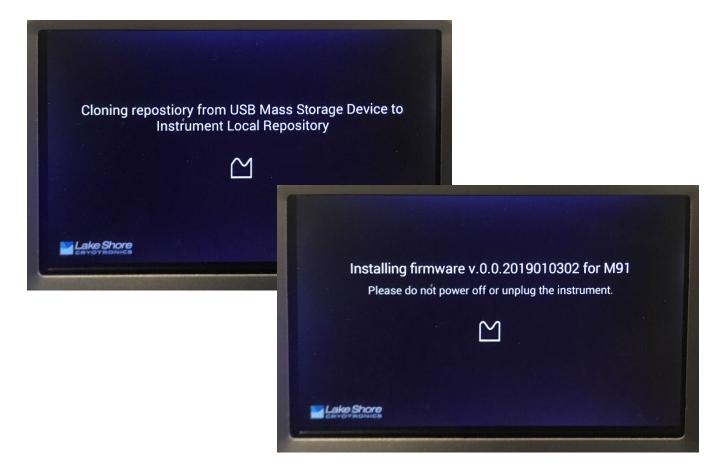
6. When complete, the instrument will return to its home screen and be fully functional again. Remove the USB flash drive, otherwise the operating system will be reinstalled every time the instrument boots up.
