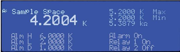
Press any of the 4 input buttons (A, B, C or D) to view or change the parameters for each channel in the input display mode
