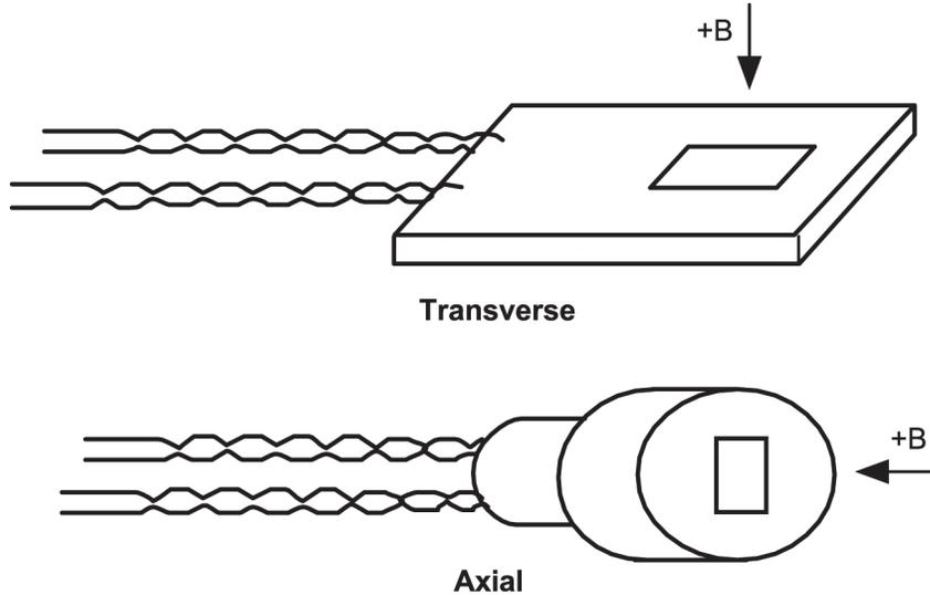
Figure 3-1. Typical Transverse and Axial Hall Sensors
