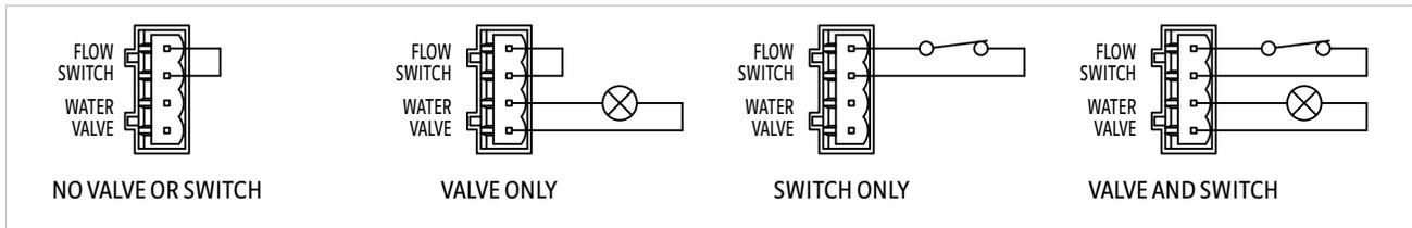
FIGURE 3-10 Typical power supply connector wiring
