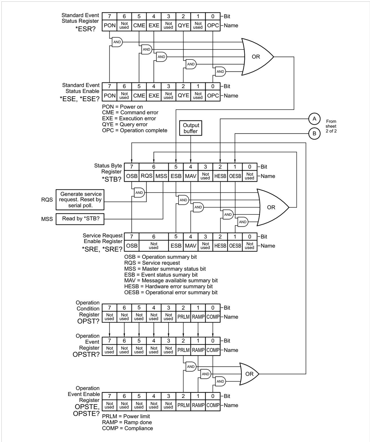
FIGURE 5-1 Model 643 status system (image 1 of 2)
