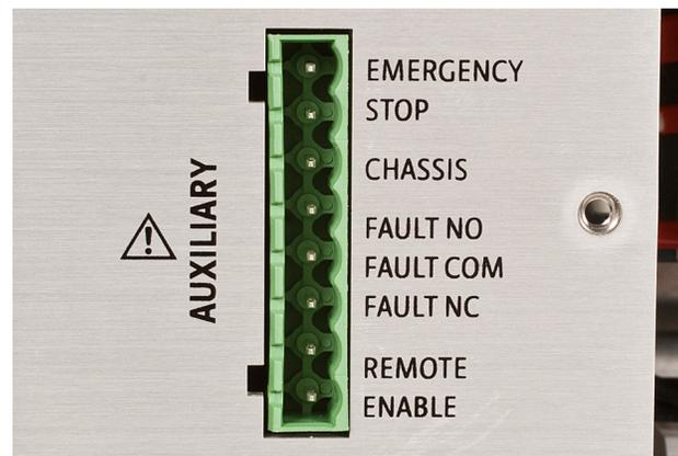
FIGURE 6-8 Auxiliary connector
