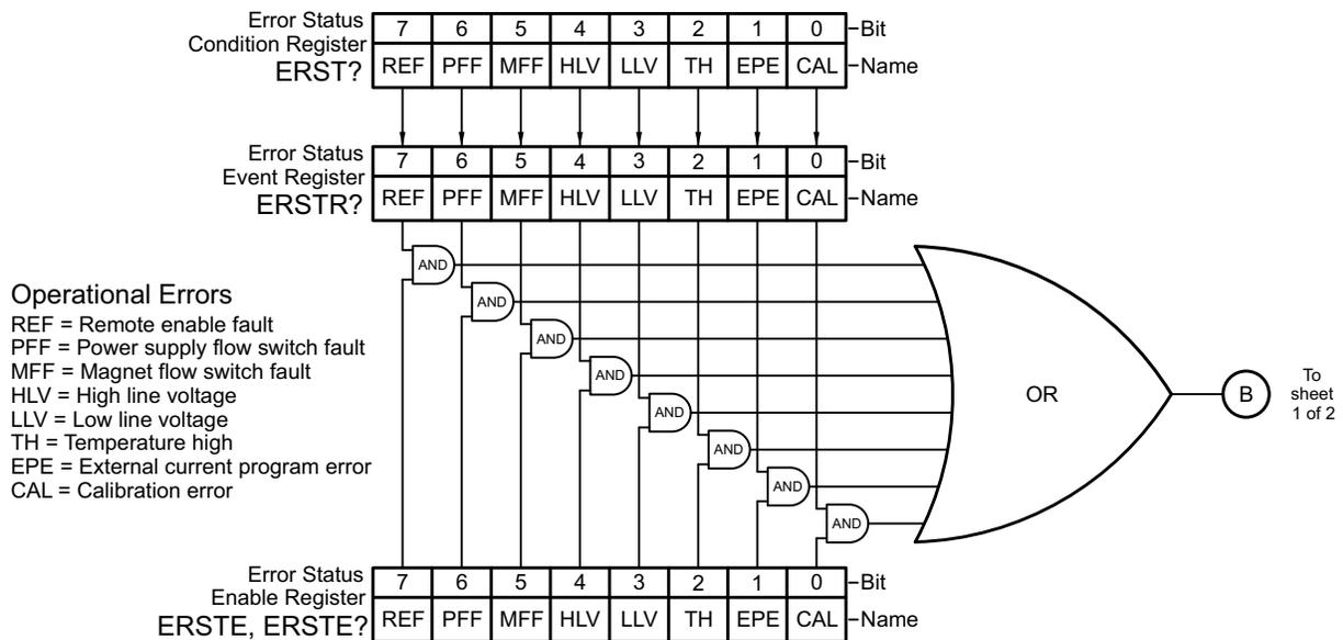
FIGURE 5-2 Model 643 status system (image 2 of 2)
