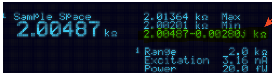
FIGURE 2-4 Display showing impedance measurement
