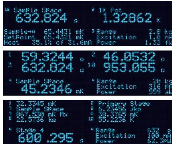
FIGURE 4-7 Model 372 screen images showing 2 (top), 4 (middle) and 8 (bottom) display locations
