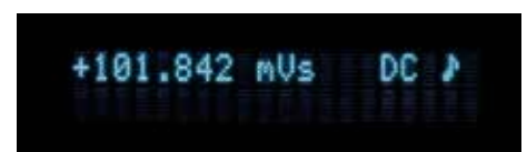
Alarm on—the alarm gives an audible and visual indication of when the flux value is selectively outside or inside a user-specified range
