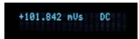
Normal reading—the default mode with the display of the live DC flux reading
