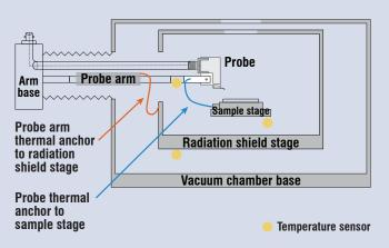
Lake Shore TTPX probe stations take thermal management to the next level with complete thermal anchoring. Plus, vapor-cooled shielding blocks radiation from reaching the sample.
