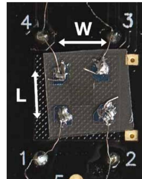
means that the phase errors for the high resistance sample are large. Using the quadrature signal as well as the in phase signal, the Hall resistance is corrected for the phase error to  $970 \Omega$ . It's important to note the Hall resistance measured with the AC method is 1% of the DC Hall resistance. The mobility for this measurement is  $0.1 \text{ cm}^2/(\text{Vs})$  – more in line with the expected results.
