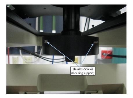
5. Attach the sample tail guide assembly you made in step 1 to the stainless steel set screws. You should feel no binding during the installation.
