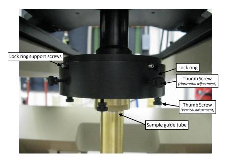
6. Visually center the ring and tight the horizontal positioning thumb screws.
