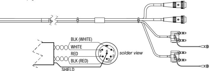
Sensors and heaters can easily be soldered to the wires at the bare end of the cable assembly. If additional reach is required between sensors or heaters, cable ties may be cut free to allow more freedom with the individual cables.
