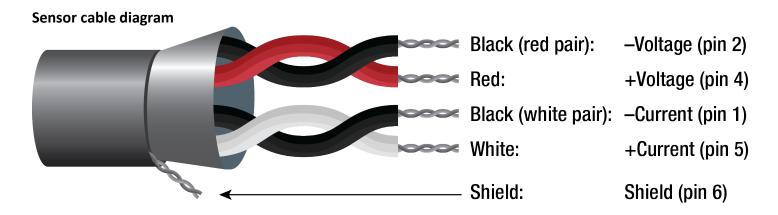
**Please note:** Previous versions of these cables used a 6-wire (3 twisted pair) cable for each sensor connection. These wire allocations were used:
