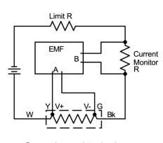
Germanium resistor basic measuring circuit
