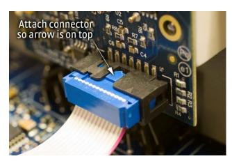
Figure 3. Proper orientation of the ribbon cable connector plug
