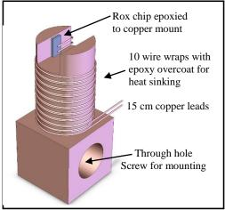
There are three aspects of temperature sensor use critical to optimum performance: mounting the sensor package, joining sensor lead wires to connecting wires, and thermally anchoring wires. Adhere to instructions below for maximum sensor performance.
