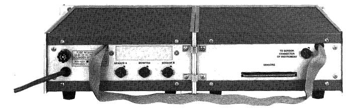
FIGURE 3.5 Model DRC-80 and SW-10A Rear View showing RM-3H Rack Mounting Hardware and Umbilical Cord Connections.
