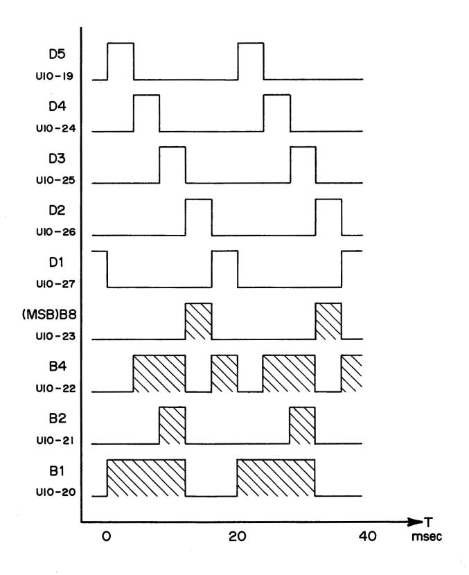
Figure 5.1 DRC-80 A/D Typical Output Signals
