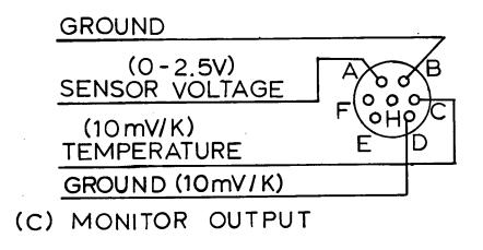
FIGURE 2.1 Sensor, Cable, and Monitor Connections
