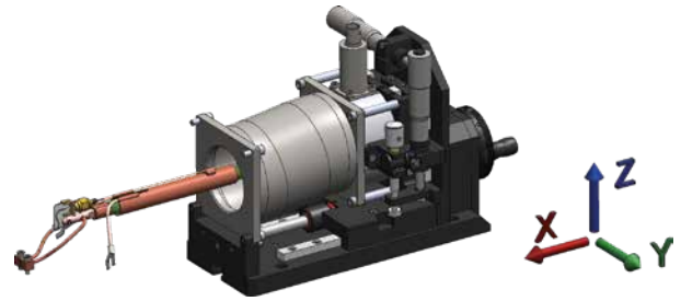
The ZN50 probe base incorporates a pair of copper braids that anchor to the sample stage to dynamically cool/heat the probe to the sample temperature
