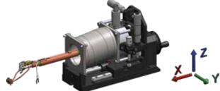
The ZN50 probe base incorporates a pair of copper braids that anchor to the sample stage to dynamically cool/heat the probe to the sample temperature
