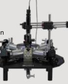
The PS-100 comes preconfigured for sensitive, high-impedance DC measurements for use in a variety of applications. It features a four-arm triaxial configuration for four-point probing and operates over a 4.2 K to 475 K temperature range. High-precision, micro-manipulated stages ensure accurate probe tip placement, and it holds samples up to 32 mm (1.25 in) in diameter.
