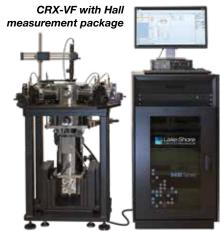
**Direct and derived measurements** as a function of field and temperature Hall voltage I-V curve measurements Resistance Magnetoresistance Magnetotransport Hall coefficient Hall mobility Anomalous Hall effect (AHE) Carrier type/concentration/density Van der Pauw and Hall bar structures
