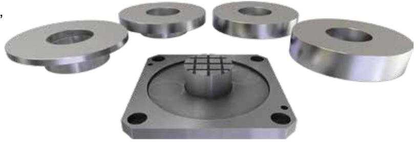
The magnets are positioned 1 mm above the top of the sample holder, creating nominal fields of 0.19 T, 0.177 T, 0.144 T, and 0.085 T at the sample holder elevation. The actual magnetic field obtained will depend on the magnet temperature. Standard operating temperature ranges for the probe station apply.
