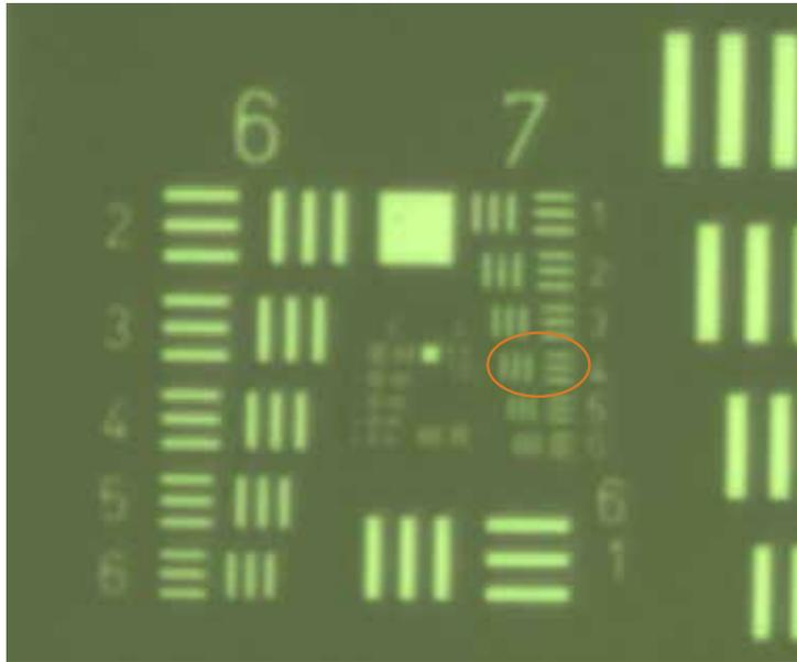
Left: smallest feature visualized (approximately 3 µm) obtained with standard 7:1 microscope and coaxial light on a CPX-VF probe station
