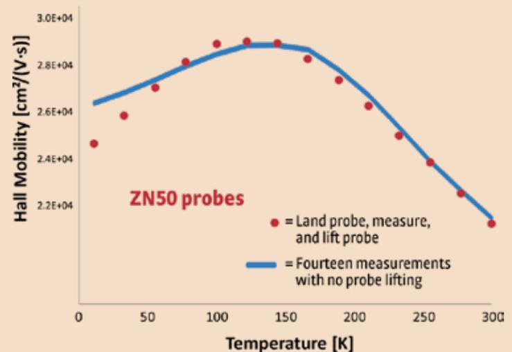
With patented ZN50R-CVT probes you don't have to constantly lift and re-land during measurements
