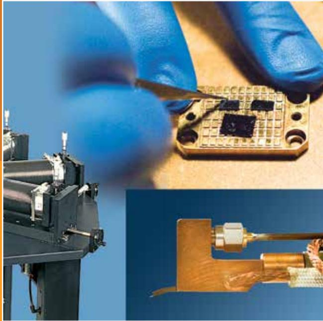
Lake Shore's cryogenic probe stations provide precisely controlled environments for non-destructive measurement of the electrical properties of materials and early-stage electronic devices.
