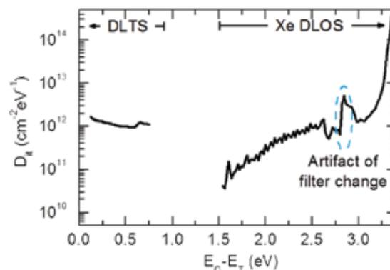
Figure 2: Interface state density ( $D_{it}$ ) at the ALD  $\text{Al}_2\text{O}_3$ /GaN interface in Figure 1 is shown using thermally-based DLTS for states within 0.8 eV of the GaN conduction band and optically stimulated emission-based DLOS using a xenon (Xe) lamp for mid-gap to GaN valence band.
