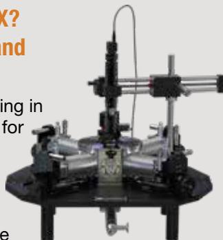
The PS-100 comes preconfigured for sensitive, high-impedance DC measurements for use in a variety of applications. It features a four-arm triaxial configuration for four-point probing and operates over a 4.2 K to 475 K temperature range. High-precision, micro-manipulated stages ensure accurate probe tip placement, and it holds samples up to 32 mm (1.25 in) in diameter.
