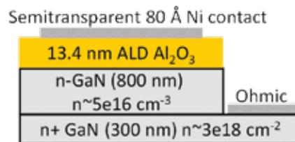
Figure 1: Metal-insulator-semiconductor structure for analyzing interface state densities at the insulator-semiconductor interface, specifically the atomic layer deposition (ALD)-grown  $\text{Al}_2\text{O}_3$ /n-type  $\text{NH}_3$ -MBE-grown GaN interface is quantified using deep level transient and optical spectroscopies (DLTS/DLOS).
