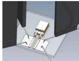
Simulates the thermal loading of a sample during probing. The PS-REF-CRX consists of a calibrated CX-1050-SD-HT-1.4M sensor chip mounted to a 10 mm × 10 mm × 0.45 mm thick sapphire substrate with landing pads. There are no leads to the sensor;
