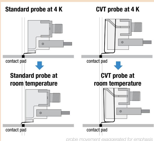
In a comparison between standard ZN50R probes and the CVT probes, you can see that the standard probes would need to be repositioned before the arms expand enough to move them off the landing position. The CVT probes flex and maintain contact with the desired location.
