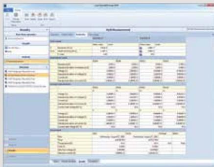
It includes all the instrumentation and data acquisition/analysis software for facilitating Hall voltage, Hall coefficient, Hall mobility, resistance, I-V curve, and other measurements.
