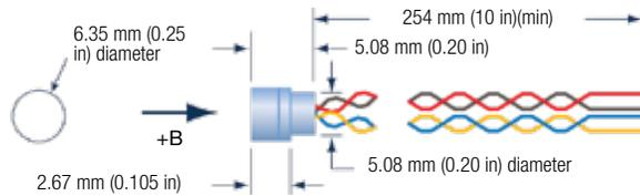
\*The active area is symmetrical with the center line of the assembly and is located 0.9 mm (0.035 in) ± 0.3 mm (0.012 in) behind the front surface of the assembly
