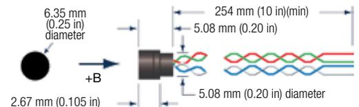
\*The active area is symmetrical with the center line of the assembly and is located approximately 0.030 in behind the front surface of the assembly
