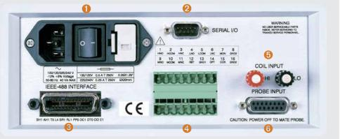
\* The Model 480 terminal block has connections for external reset. With this feature. a foot pedal or programmable logic controller (PLC) can be used to start a new measurement cycle. The external reset is TTL-compatible and a logic low will activate a reset. The signal is internally pulled up to allow operation with a simple switch closure between pins 12 and 13.
