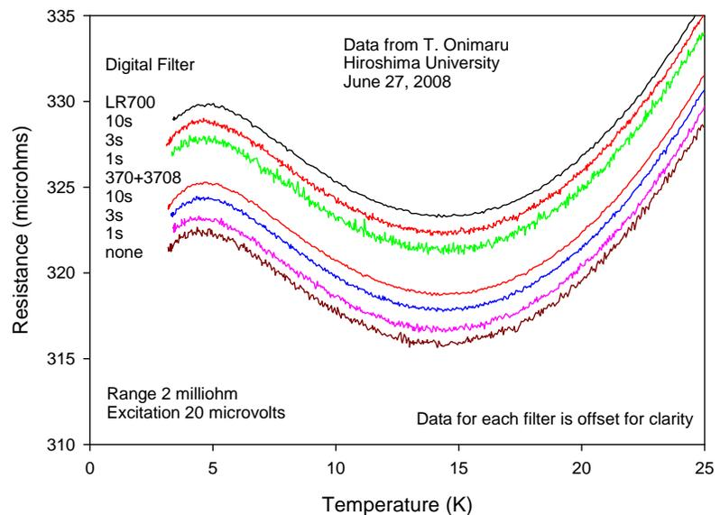
**Figure 1: Comparison of Lake Shore Model 370 AC resistance bridge with Model 3708 preamp/scanner and Linear Research Model LR700 AC resistance bridge**
