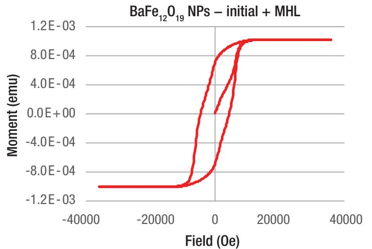
Figure 6: Initial magnetization curve and MHL for a BaFe<sub>12</sub>O<sub>19</sub> permanent magnet sample
