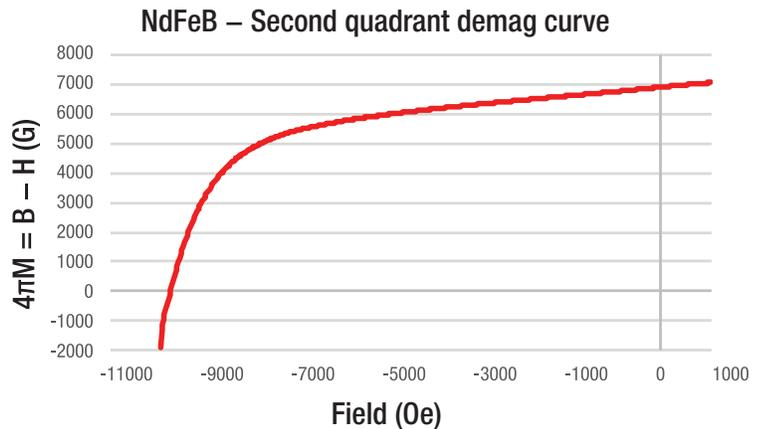
Figure 3: Second quadrant demagnetization curve for a NdFeB permanent magnet sample
