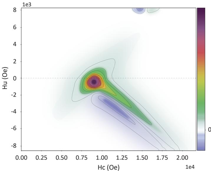
Figure 5: 2D FORC diagram for a NdFeB permanent magnet sample
