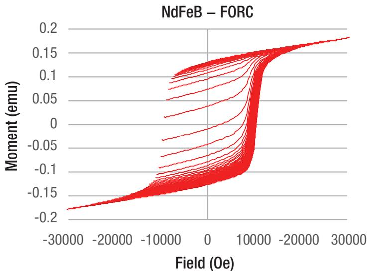
Figure 4: Measured FORCs for a NdFeB permanent magnet sample
