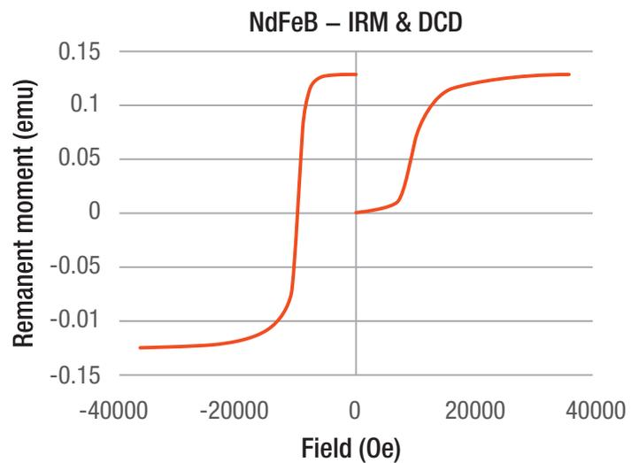
**Figure 2:** IRM and DCD remanence curves for a NdFeB permanent magnet sample
