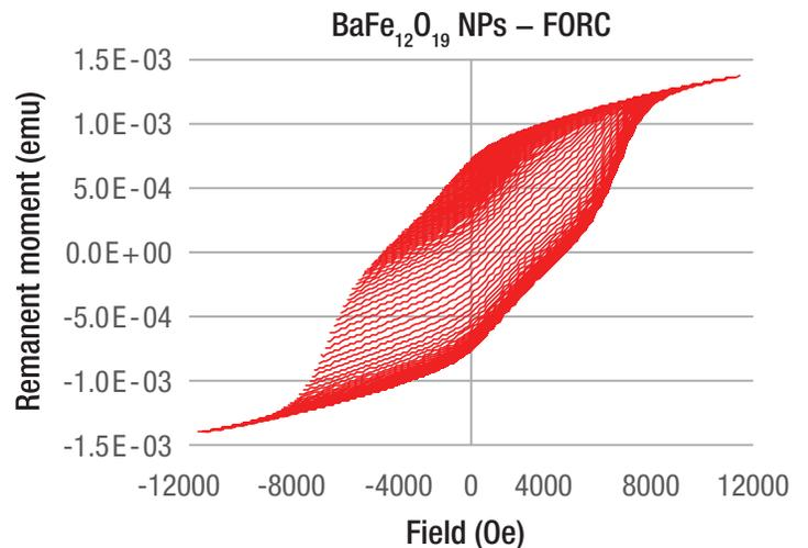
Figure 8: Measured FORCs for a BaFe<sub>12</sub>O<sub>19</sub> permanent magnet sample
