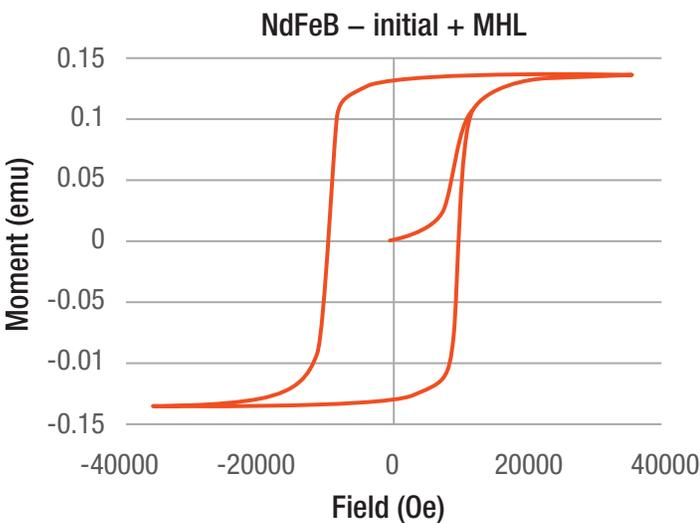
**Figure 1:** Initial magnetization curve and MHL for a NdFeB permanent magnet sample
