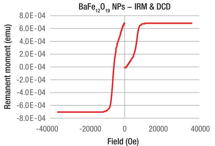
Figure 7: IRM and DCD remanence curves for a BaFe<sub>12</sub>O<sub>19</sub> permanent magnet sample
