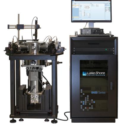
In addition to the 8400 Series software, the system includes all the hardware necessary for probe station-based measurements: a vertical field superconducting magnet, a closed-cycle refrigerator, a Model 336 temperature controlller, a vacuum turbopump, a separate monitor (not shown) for examining magnified samples, and more. For a complete list of contents, see www.lakeshore.com.
