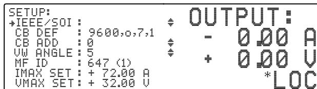
Use the Cursor keys to move the line indicator up or down. The up and down arrow icon indicates parameters that can only be changed with the up or down Numeric Entry keys. All others can be changed using all the numeric entry modes, including the cursor. Below are valid Setup entries:
