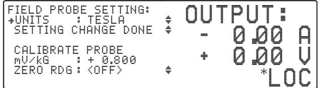
The cursor up and down keys move the line indicator (→). The up and down arrow icon indicates parameters that can only be changed using the Data Entry up and down arrows.
