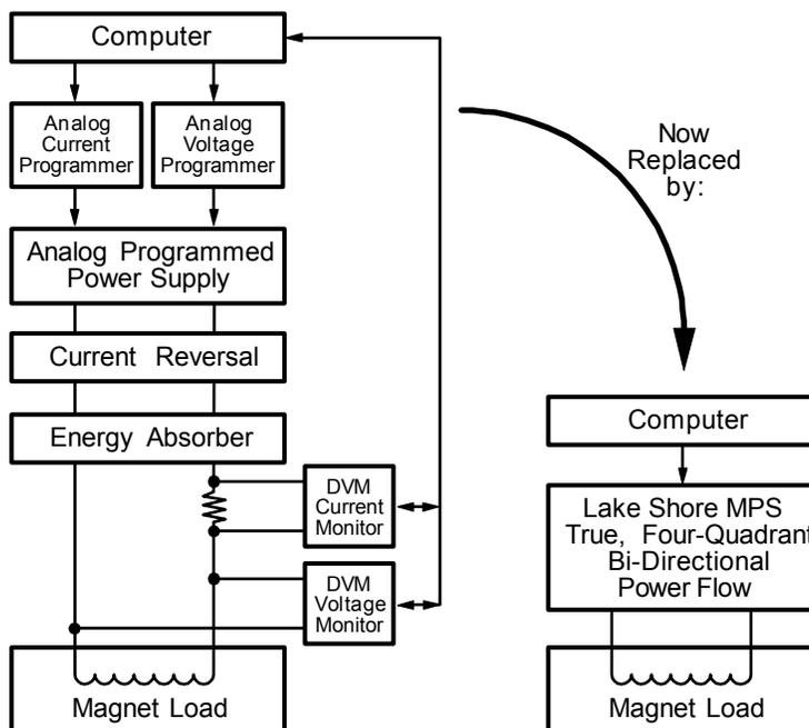
Figure 1-2 Comparison of Old and New MPS Designs
