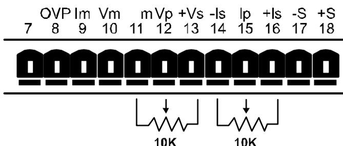
**Figure 2-3** Analog Monitoring , Programming, & Remote Sense Connections
