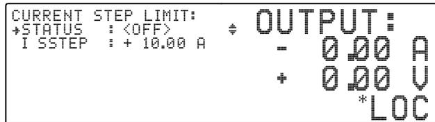
Use the Cursor keys to move the line indicator up and down. The ⚡ icon indicates parameters that can only be changed using the up or down Numeric Entry keys. Change all others using all the numeric entry modes, including the cursor. (See Section 3 for keypad operations.) Below are valid Output Current Step Limit entries:
