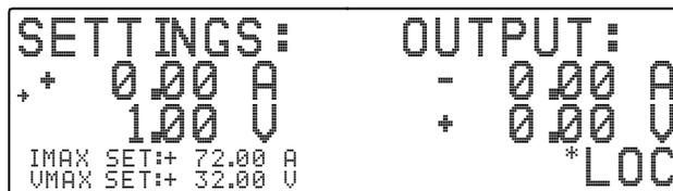
The OUTPUT screen indicates the output values and the interface status. The Normal Display key returns the display to this screen at any time.
