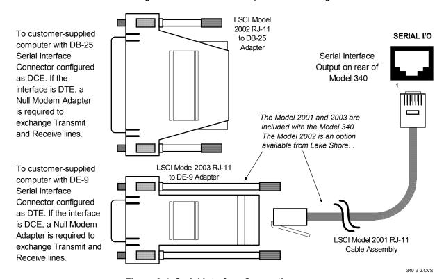
Figure 9-4. Serial Interface Connections
