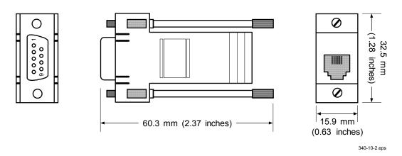
Figure 10-2. Model 2003 RJ-11 to DE-9 Adapter
