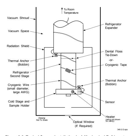
Figure 2-2. Typical Sensor Installation In A Mechanical Refrigerator
