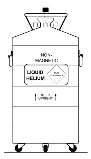
Figure 3-1. Typical Cryogenic Storage Dewar
