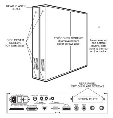
Figure 10-5. Cover and Option Plate Screws
