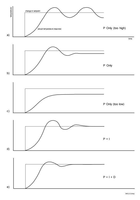
Figure 2-3. Examples of PID Control
