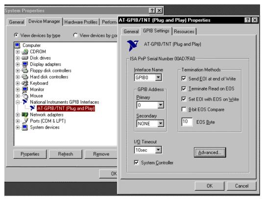
Figure 9-1. GPIB Setting Configuration
