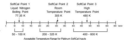
**Point 1:** Calibration data point at or near the boiling point of nitrogen (77.35 K). Temperatures outside 50 K to 100 K are not allowed.
