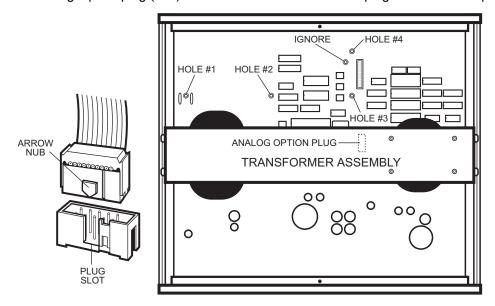
Figure 10-6. Model 340 Mounting Holes and Analog Option Plug
