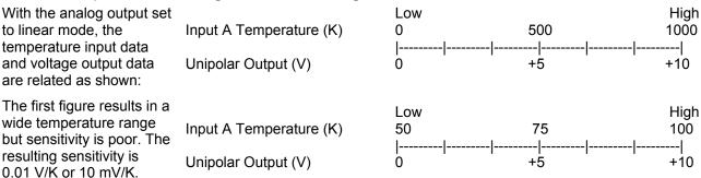
If the application does not require a wide temperature range, the user can change the value of the low and high parameters to improve sensitivity. This setup has a narrow range with much improved sensitivity of 0.2 V/K or 200 mV/K. Please note that in any application, the resolution of the analog output voltage is always 1.25 mV as specified.
