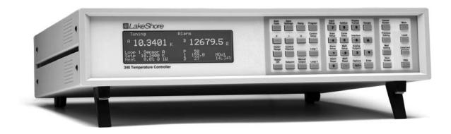
1The Lake Shore SoftCal™ algorithm for silicon diode and platinum RTD sensors is a good solution for applications that need more accuracy than a standard sensor curve but do not warrant traditional calibration. SoftCal™ uses the predictability of a standard curve to improve the accuracy of an individual sensor around a few known temperature reference points.
