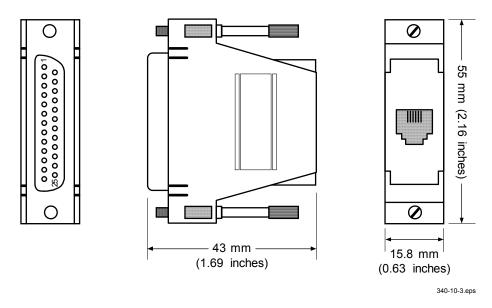
Figure 10-3. Optional Model 2002 RJ-11 to DB-25 Adapter
