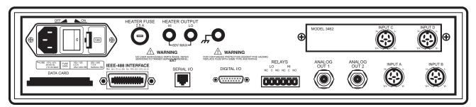
Figure 10-8. Model 340 Rear Panel with Model 3462 Option Card Installed
