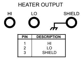
Figure 11-8. HEATER OUTPUT Rear Panel Connector Details
