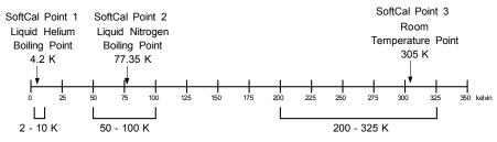
Acceptable Temperature Range for Silicon Diode SoftCal Inputs
