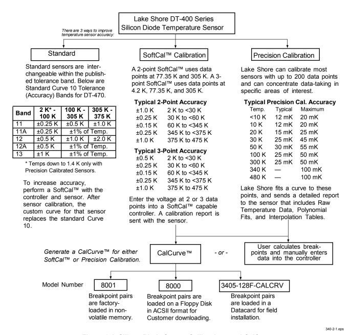
Figure 2-1. Silicon Diode Sensor Calibrations and CalCurve
