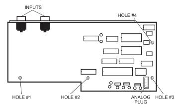
Figure 10-7. Mounting Holes & Analog Plug
