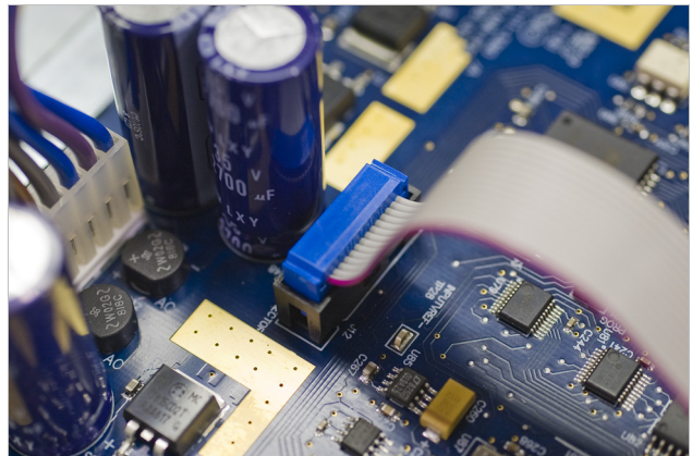
FIGURE 7-3 Proper orientation of the ribbon cable connector plug
