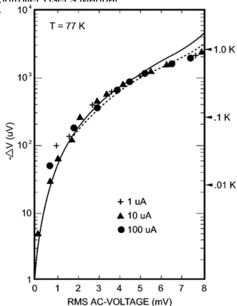
**FIGURE 4.** DC offset voltage as a function of rms ac voltage across a silicon diode temperature sensor operating at 77 K. The symbols represent data recorded at three different dc operating currents with a 60 Hz signal superimposed. The solid curve gives small signal model results while the dashed curve represents the extended calculations. Equivalent temperature errors are indicated along the right edge.
