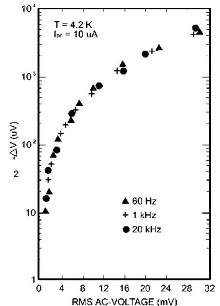
**FIGURE 7.** DC offset voltage as a function of rms ac voltage across a silicon diode temperature sensor operating at 77 K. The symbols represent data recorded at a 10  $\mu$ A dc current with the ac current modulation at 60, 1000, and 20,000 Hz.
