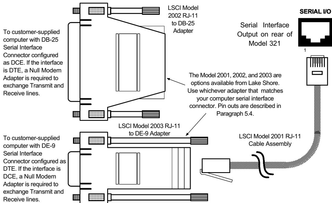
Figure 4-1. Optional Serial Interface Connections
