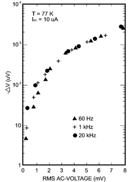
**FIGURE 6.** DC offset voltage as a function of rms ac voltage across a silicon diode temperature sensor operating at 77 K. The symbols represent data recorded at a 10  $\mu$ A dc current with the ac current modulation at 60, 1000, and 20,000 Hz.
