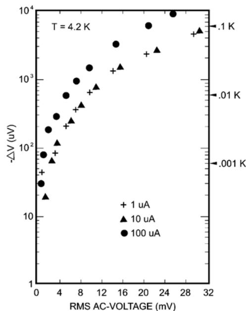
**FIGURE 5.** DC offset voltage as a function of rms ac voltage across a silicon diode temperature sensor operating at 4.2 K. The symbols represent data recorded at three different dc operating currents with a 60 Hz signal superimposed. Equivalent temperature errors are indicated along the right edge.
