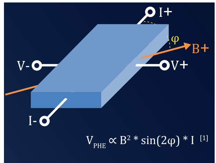
**Figure 1:** Planar Hall effect produces an unwanted Hall voltage when the field is in plane with the sensor.
