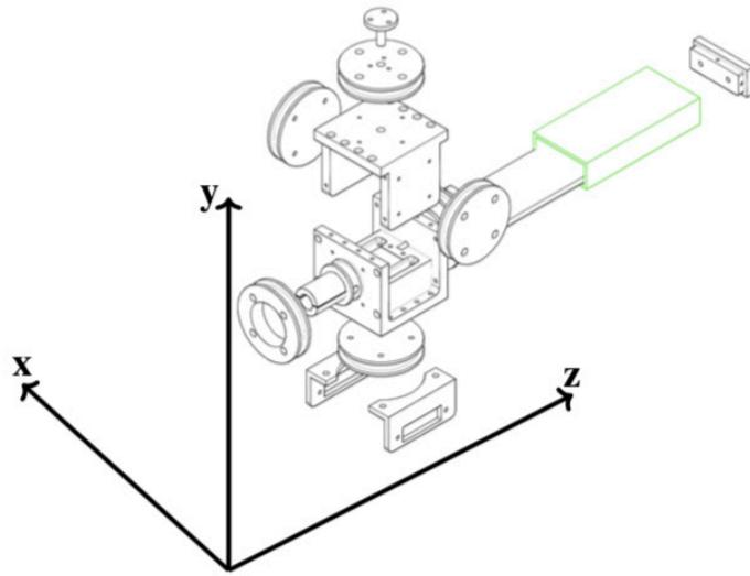
**Figure 2:** The experimental setup used to test the Hall sensor. The box containing the sensor is attached to the 2 K stage of a pulse tube cooler (PTC), as shown in the photograph on the left. The exploded image of the box is shown on the right with the axis directions indicated. The Hall probe is mounted in the square region in the center, where the detector chip will sit during testing.
