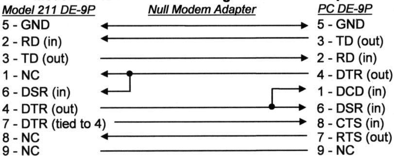
**NOTE:** Same as null modem cable design except PC CTS is provided from the Model 211 on DTR.
