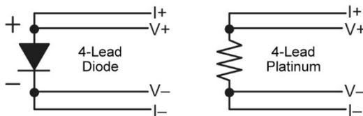
In a 4-lead measurement, current leads and voltage leads run separately to the sensor. With separate leads, there is little current in the voltage leads so their resistance does not enter into the measurement. Resistance in the current leads will not change the current as long as the voltage compliance of the current source is not reached. When 2-lead sensors are used in 4-lead measurements, the short leads on the sensor have an insignificant resistance.
