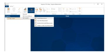
In the left hand pane, when the start button is pressed, a sequence of measurement functions are executed in order. By selecting each step independently, the user can edit the step parameters to control the measurement execution.
