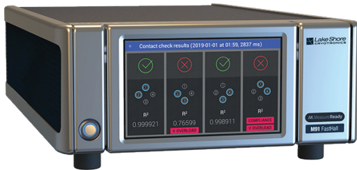
The M91 automatically checks and graphically displays sample contact quality
