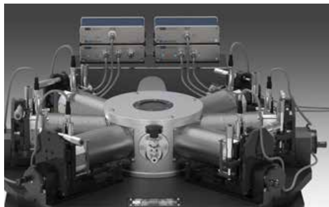
The SMU-10 enables I-V characterization of nanometer-scaled and atomically thin devices using voltage or current control — from DC to 100 kHz, with or without AC modulation.
