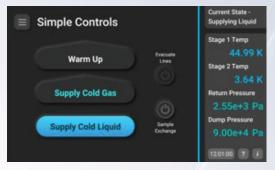
A single button controls system cooldown and adjusts valves automatically, allowing you to be up and running fast.
