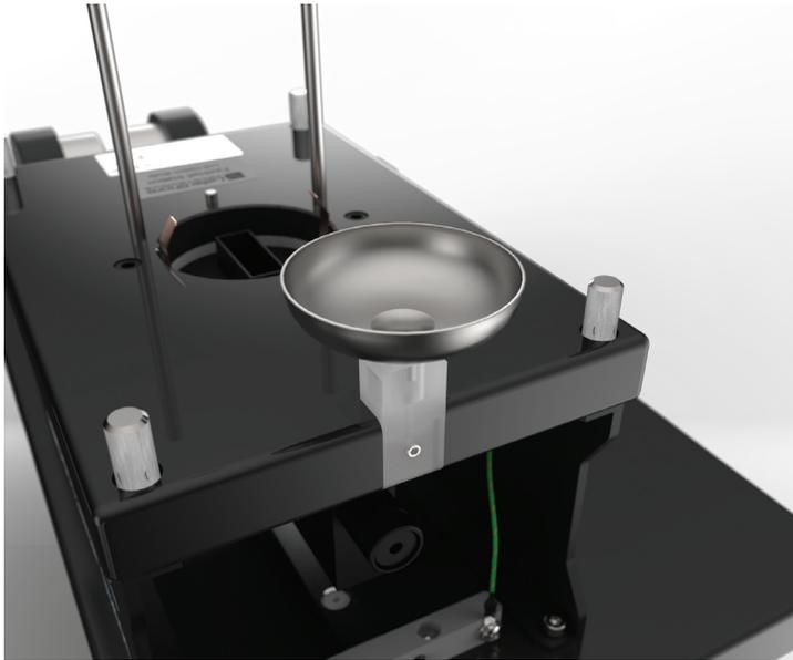
The LN<sub>2</sub> option includes a sample platform with a reservoir and funnel for measurements in a LN<sub>2</sub> bath.
