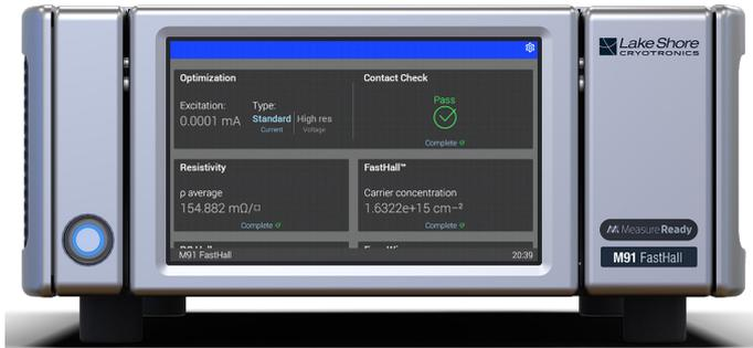
FastHall eliminates the need for field reversal Up to 100× faster for low-mobility materials Lower mobilities can be measured using lower fields.
