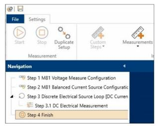
Create nested, multi-level measurement loop sequences with drag-and-drop controls, and coordinate the cryostat environment with electrical source sweeps and multi-channel data collection
