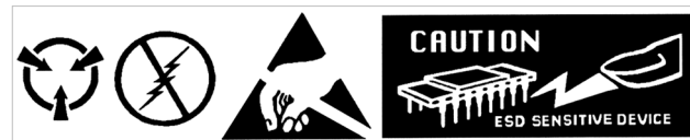
FIGURE 7-1 Symbols indicating ESD sensitivity
