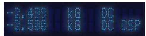
The display configured to show the field control setpoint and current field value, when field control is active
