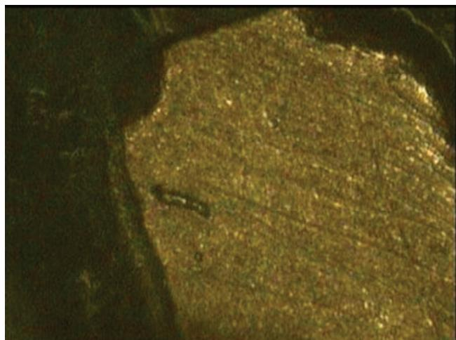
Figure 5 Contact pad after probe tip is removed
