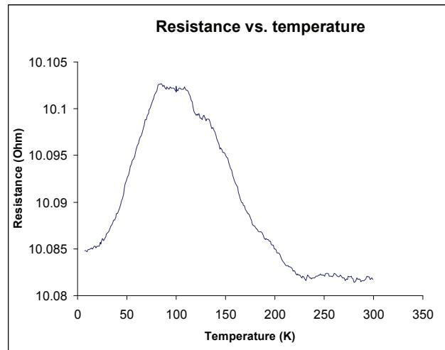
Figure 1 Variable temperature measurement of a 10  $\Omega$  resistor
