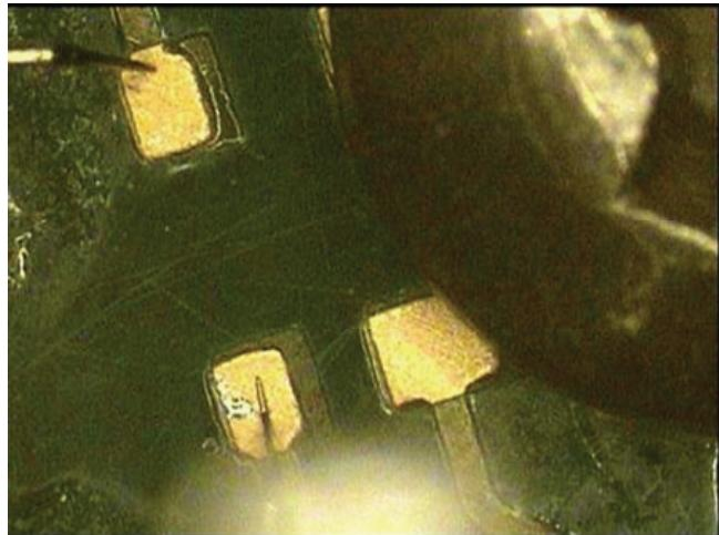
Figure 2 Probes positioned on measurement pads;
