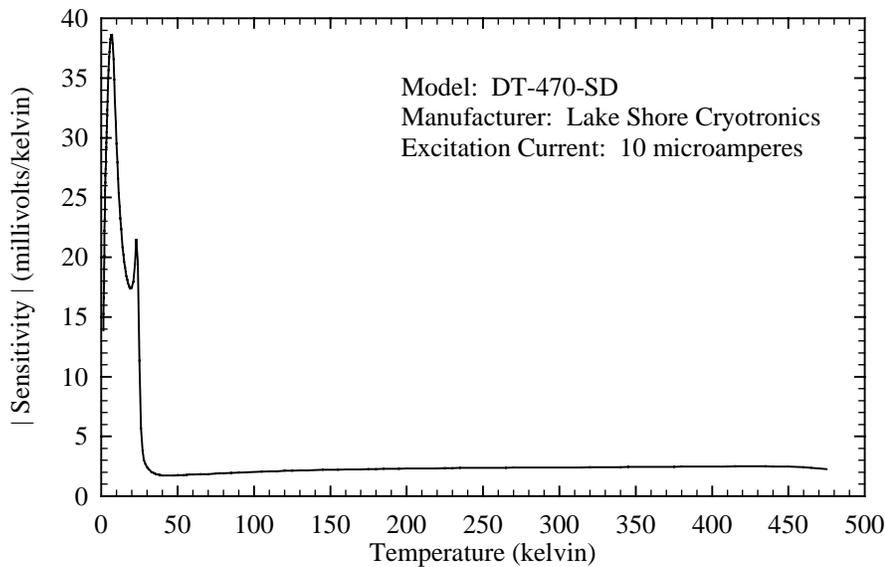
**FIGURE 2.** Typical temperature sensitivity as a function of temperature for a typical cryogenic diode thermometer excited at 10  $\mu$ A. (Data shown is for a Lake Shore model DT-470-SD cryogenic diode thermometer.)
