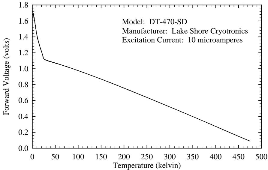
**FIGURE 1.** Typical forward voltage as a function of temperature for a typical cryogenic diode thermometer excited at 10  $\mu$ A DC. (Data shown is for a Lake Shore model DT-470-SD cryogenic diode thermometer.)
