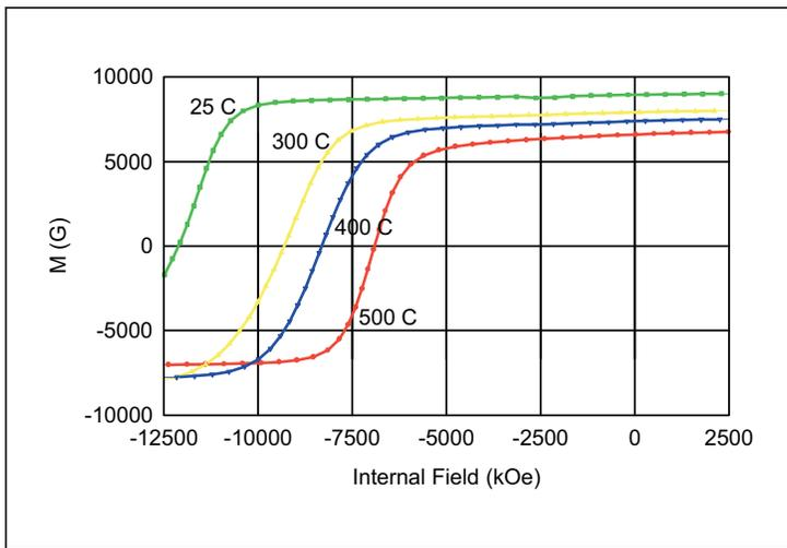
Figure 4  $M(H,T)$  curves for the SmCo magnet material.
