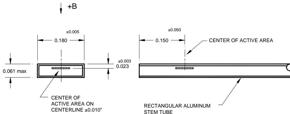
Note that the “active area” of the probe is closer to one side. This side should be nearest to the mass standard during measurement. An easy method of insuring that this is the case is to position the Lake Shore logo on the probe handle towards the weight.
