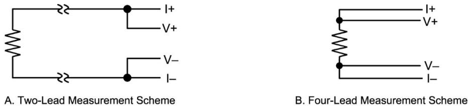
**Figure 1. Two-Lead Versus Four-Lead Measurements**
