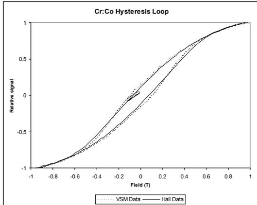
Figure 2 Hysteresis loop with minor loop for Cr:Co sample. Both VSM data and AHE data are shown. The data has been normalized to one.
