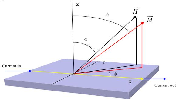
Figure 1. Geometry of the AHE measurement.  $\alpha$  is the angle between the applied field and the normal to the sample,  $\theta$  is the angle between the magnetization and the normal, and  $\phi$  is the angle between the current and the in plane component of the magnetization.
